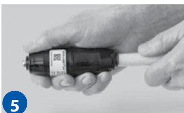
5 Stab tubing into the coupling until it bottoms out.
