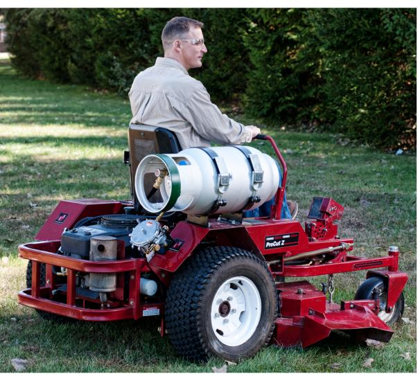
AltFuel Green conversion kits retrofit 4 stroke carbureted gasoline engines to run on clean, safe, and efficient propane fuel.
