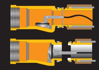
The Smart-Hose Break-Away has been designed to protect your plant's piping and bulk-head from pull-away incidents. Designed to integrate with the Smart-Hose safety system and engineered with a predetermined break-point. The Smart-Hose Break-Away can add an additional layer of protection inside your plant and trans-port hoses while protecting your facility from the devastating consequences of a pull-away accident.
